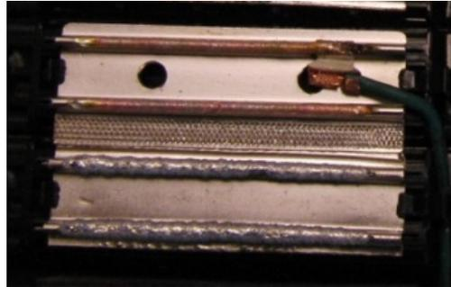
**Figure 28 – Two types of bus bars ultrasonically bonded in the center to each other**
